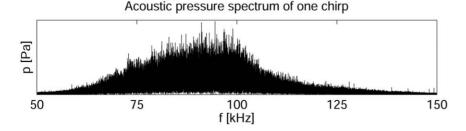
Figure 3. Acoustic power spectrum of one chirp. doi:10.1371/journal.pone.0026476.g003
