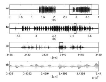
**Figure 4. The time course of the male's ultrasonic courting song.** a) two chirps separated by a silent period, b) a detail of one chirp, c) a detail of one modulation cycle, d) individual clicks. doi:10.1371/journal.pone.0026476.g004
