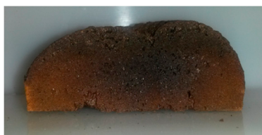
Figure 20. Cross-sectional picture of TETM/DDS/expandable microspheres foam, cured according to the C 2 cycle (length = 7 cm).
