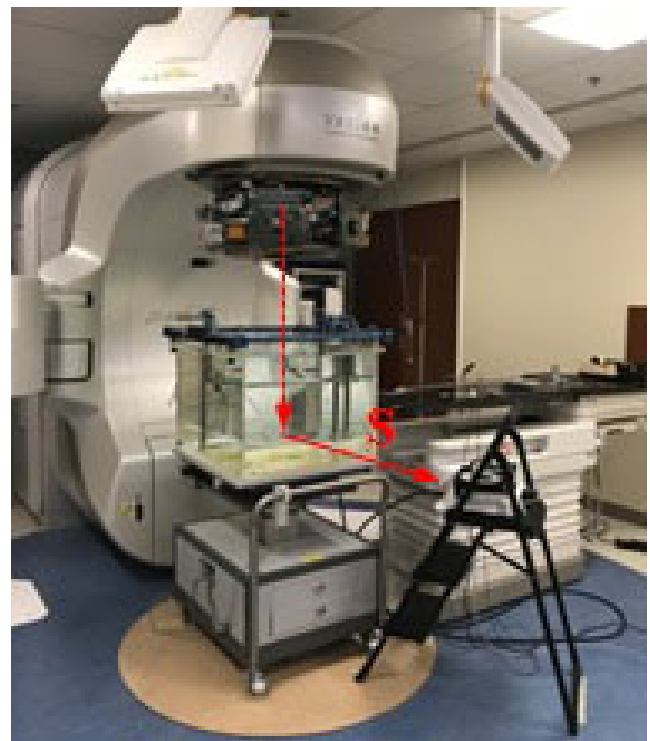
Fig. 1. Setup of the Common Control Unit (CCU) during the data measurement. The CCU was placed on a stand at 82 cm above the floor. The stand was then positioned at various distances S from the radiation beam. S is the distance between the rear edge of the CCU and the radiation beam central axis. The geometries used to measure the data were gantry = 0^\circ , collimator = 0^\circ , and SSD = 100 cm.
