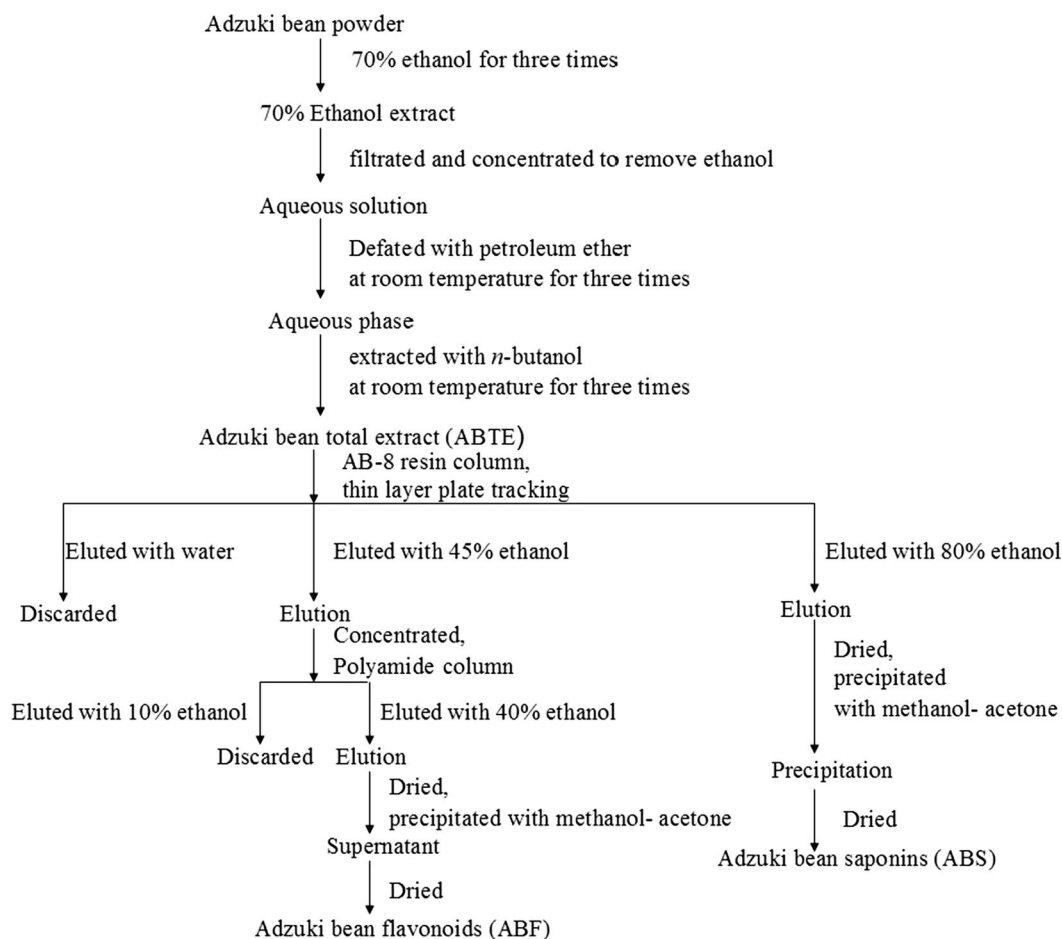
Fig. 1 Extraction and isolation scheme of total extract, flavonoids and saponins from adzuki bean
