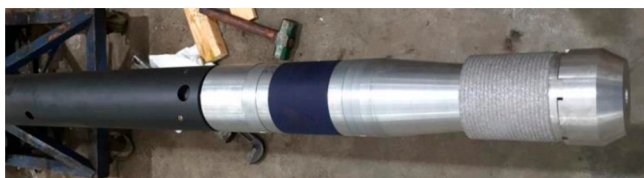
Figure 21. Baker Hughes SPECTRE fully soluble fracturing bridge plug. Reprinted with permission from ref 154. Copyright 2019 Journal of Yangtze University(Natural Science Edition).
