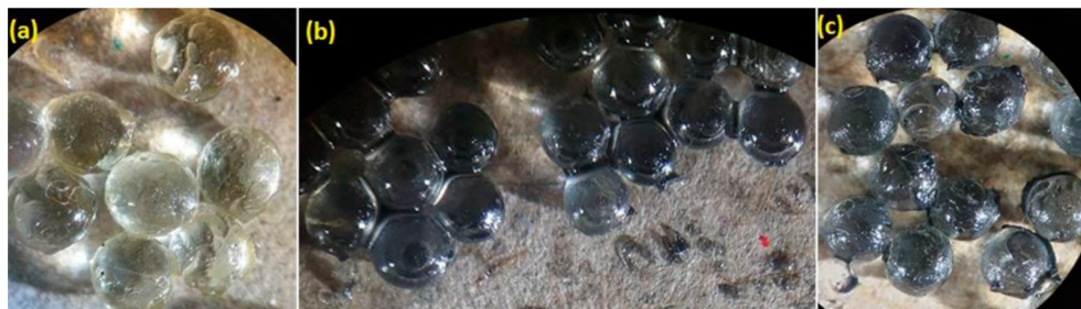
Figure 14. (a) Glass bead urethane-coated proppant containing 0.1% CNTs. (b) Glass bead urethane coated containing 0.5% CNTs. (c) Glass bead urethane-coated proppant containing 1% CNTs. Reprinted with permission from ref 133. Copyright 2022 Springer.
