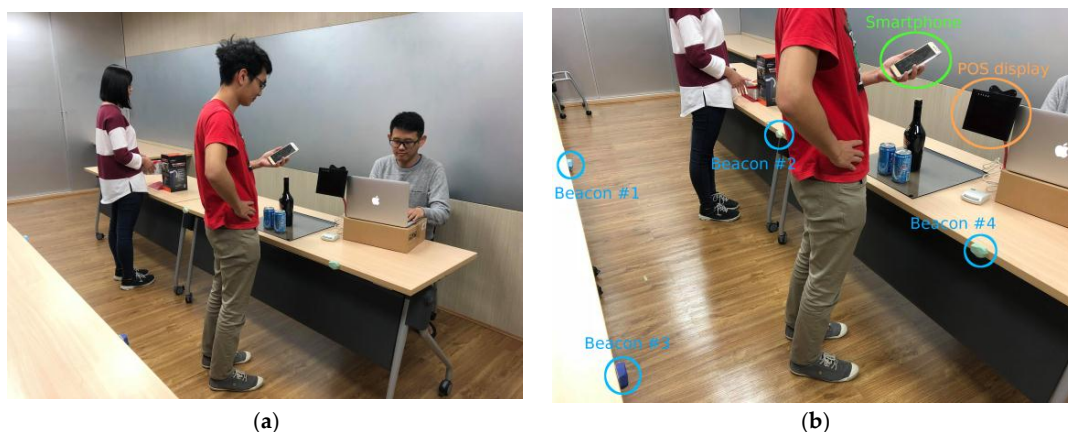
Figure 6. The practical implementation of the proposed mobile payment system: (a) four Bluetooth beacon tags are placed at the same height horizontal surface; and (b) a closer look on the arrangement of each device.
