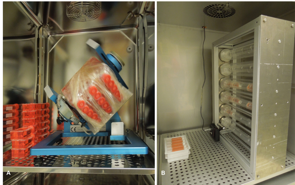
Fig 1. A: Random Positioning Machine (RPM) and B: 2D-Clinostat.
