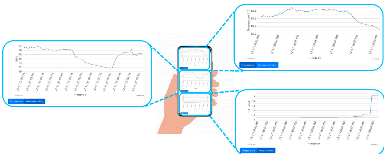
Figure 9. Simultaneous acquisition of ambient temperature and ambient relative humidity (RH) of the greenhouse node and soil water content of a single plant node, shown on the display of a portable device.
