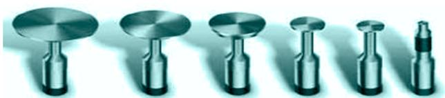
Figure 9. A variety of sizes of cones and plates are available. The larger sizes are recommended for low viscosity materials, and smaller sizes are recommended for high viscosity materials.
