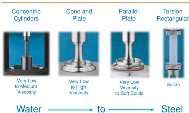
Figure 8. Geometries are available for rotational rheometers.
