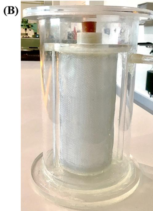
**Figure 6.** (A) Schematic diagram of the radial-flow tubular MBR and (B) photo of the assembled tubular MBR.
