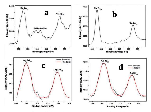
**Figure 16.** XPS spectra of Cu2p (**a**) before and (**b**) after sputtering, and Ag3d (**c**) before and (**d**) after sputtering, in Ag<sub>shell</sub>Cu<sub>core</sub> nanoalloy. Reproduced with permission from Reference [262]. Copyright 2015, Royal Society of Chemistry.
