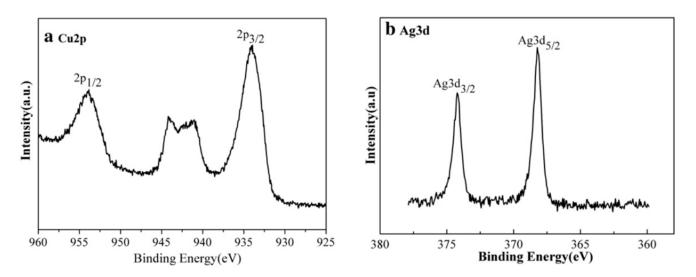
**Figure 15.** XPS spectra of (**a**) Cu2p and (**b**) Ag3d in AgCu<sub>2</sub>O nanoalloys. Reproduced with permission from Reference [242]. Copyright 2015, Elsevier.
