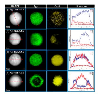
**Figure 18.** TEM-EDXS in high-angle annular dark field (HAADF) mode analysis of four different types of distribution of Ag and Cu in nanoalloy. Red arrow on HAADF image is the position and direction of line scan. Reproduced with permission from Reference [237]. Copyright 2014, American Chemical Society.
