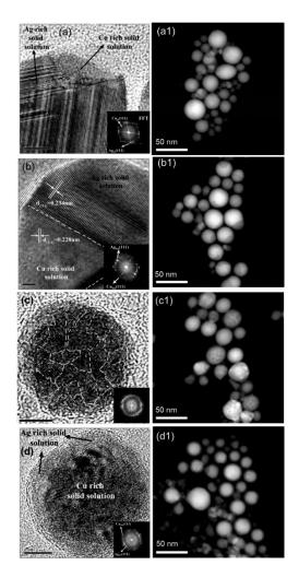
**Figure 12.** HRTEM photomicrographs of AgCu nanoalloys, showing four different microstructures: (**a**,**b**) separated phases, (**c**) nanograins and (**d**) core-shell with, respectively, four different Cu concentrations (20%, 40%, 60%, 80%). (**a1–d1**) images of four respective target compositions at low magnification. Reproduced with permission from Reference [237]. Copyright 2014, American Chemical Society.
