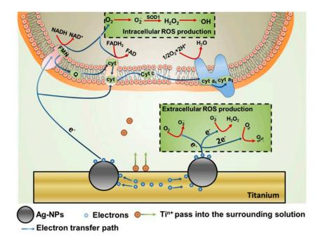
**Figure 5.** Production of ROS outside and inside bacterial cells. Reproduced with permission from Reference [80]. Copyright 2017, Elsevier.
