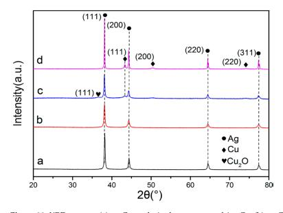
**Figure 20.** XRD spectra: (a) no Cu peaks in the spectrum of  $Ag_6Cu$ ; (b) no Cu peaks in the spectrum of  $Ag_2Cu$ ; (c) peaks of Cu and Cu<sub>2</sub>O in the spectrum of  $AgCu_3$ ; (d) peaks of Cu and Cu<sub>2</sub>O in the spectrum of  $AgCu_3$ ; (d) peaks of Cu and Cu<sub>2</sub>O in the spectrum of  $AgCu_3$ . Reproduced with permission from Reference [272]. Copyright 2019, American Chemical Society.
