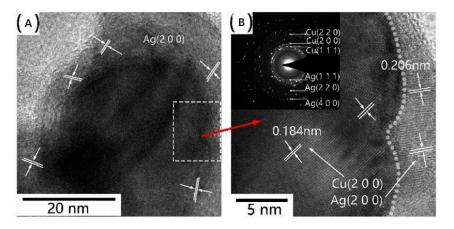
**Figure 17.** (**A**) HRTEM image of core-shell microstructure, in which Cu is the core, and Ag the shell; (**B**) magnified HRTEM image. Reproduced with permission from Reference [268]. Copyright 2017, Elsevier.
