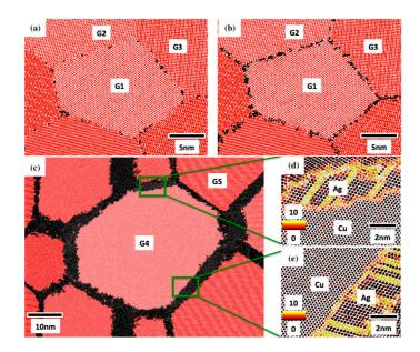
**Figure 13.** Microstructures of Ag doping Cu grain boundaries; (a-c) samples are based on the increases in Ag concentration; (d,e) are the Cu/Ag interfaces. For (a-c), red denotes Cu and black denotes Ag; for (d,e), the perfect FCC structure is marked 0, the light color, while defects are marked 10, the black color. Reproduced with permission from Reference [256]. Copyright 2017, Springer Nature.
