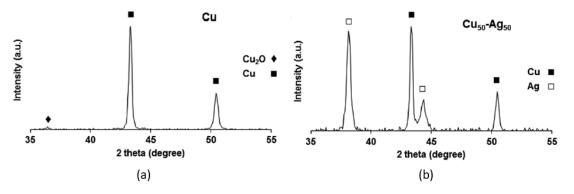
**Figure 19.** XRD spectra of (**a**) Cu NPs and (**b**) Cu<sub>50</sub>-Ag<sub>50</sub> NPs. Reproduced with permission from Reference [246]. Copyright 2016, Royal Society of Chemistry.
