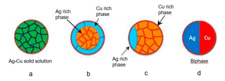
**Figure 11.** (a) Single-phase AgCu solid solution; (b) core-shell structure of AgCu nanoalloys; (c) structure of Ag and Cu in both phases; (d) biphasic. Reproduced with permission from Reference [254]. Copyright 2016, American Chemical Society.
