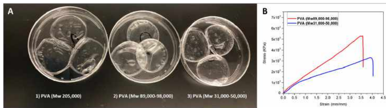
Figure S6. A) Optical photos of PVA-Hs made with different molecular weights using NaOH-induced gelation methods. B) Tensile test results for PVA-Hs with different molecular weights (sample size: 15, 5, 0.2 mm, tests speed: 20 mm/min). Both samples were immersed in water overnight and tested afterwards.
