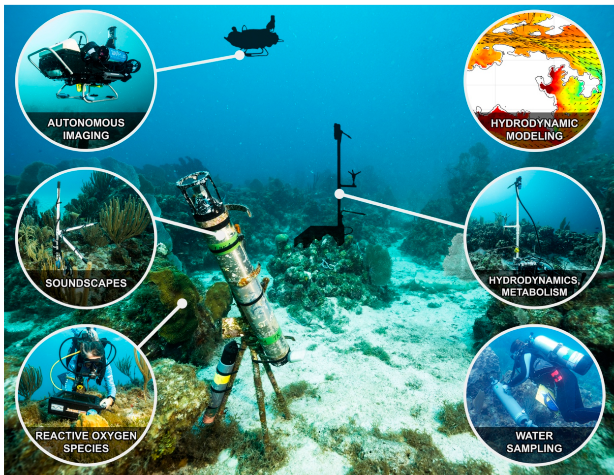
Figure 1. Conceptual diagram of case study reefs in which multiple diagnostic measures of reef health are collected in parallel by moored equipment, divers, and autonomous instruments to examine biological, chemical, and physical reef components and processes represented in Table 1. Measurements and equipment from the top right, moving clockwise, include hydrodynamics simulated using numerical models; assessment of reef metabolism using an acoustic Doppler instrument coupled to chemical sensors and hydrodynamics measured in situ using sensors, such as a Doppler current meter; water sampling using Niskin bottles (or other collection devices) to obtain samples for reef water microbes, eDNA, and metabolites; measurement of reactive oxygen species in situ using the DISCO instrument; a hydrophone to record the reef soundscape; and an autonomous vehicle capable of imaging the reef benthic and fish communities.
