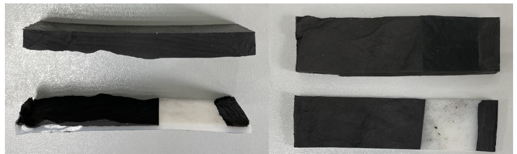
Figure 6. Cohesive nature of delamination of two-layer materials (e.g.,: elastomer/UHMWPE-TMTD).
