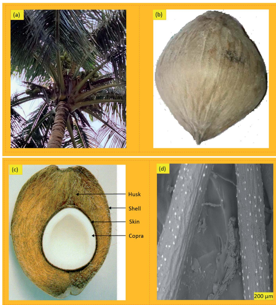
Fig. 1 Photographs showing the physical and morphological structure of coconut plants and coir fiber: (a) coconut plants in Bangladesh (digital photographs taken by Muhammad Abu Taher); (b) coconut fruits (digital photographs taken by Muhammad Abu Taher); (c) cross-section of coconut fruits; 43 (d) SEM image of coir fiber. Adapted with permission from Elsevier (c). 43 Copyright, Elsevier 2004 (c).
