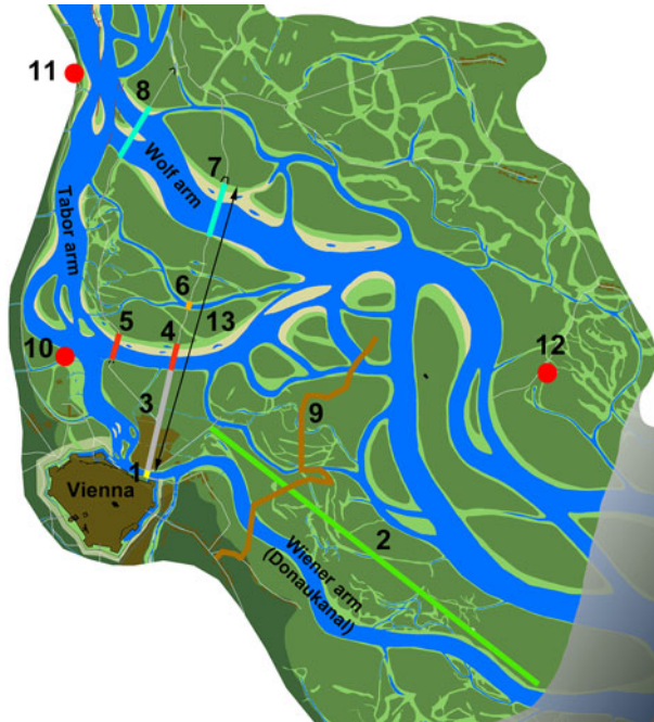
Fig. 6 Main landmarks used for the reconstruction of the riverscape in 1570. 1 Schlagbrücke , 2 Prater Main Avenue , 3 historically surveyed transect from Schlagbrücke to Tabor bridge , 4 old Tabor bridge until 1565, 5 new Tabor bridge since 1569/70, 6 Lackenbrücke , 7 old Wolf bridge until 1565, 8 new Wolf bridge since 1569/70, 9 Burgfriedsgrenze with boundary stones, 10 confluence of tributary Alserbach , 11 village Nußdorf , 12 village Stadlau , and 13 distance between inner and outer bridge based on Schmeltzl 1547/48
