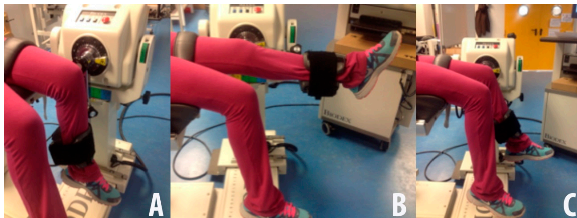
Figure 1. Isokinetic protocol, with start (maximal flexion: 90°) (A) and final (maximal extension: 10°) (B) positions; Isometric protocol (70° position) (C).
