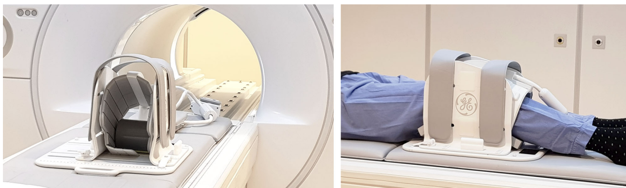
FIGURE 1: Standardized positioning of the knee during MRI. Illustrated is the positioning of the 16-channel flexible coil in combination with the support device that was used for knee stabilization and standardization of the knee flexion angle.
