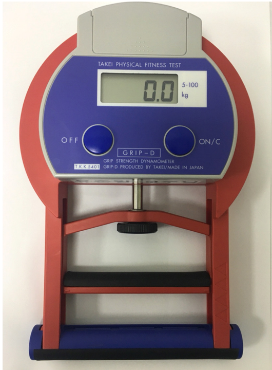
Fig. 1. Hand dynamometer used in the study.
