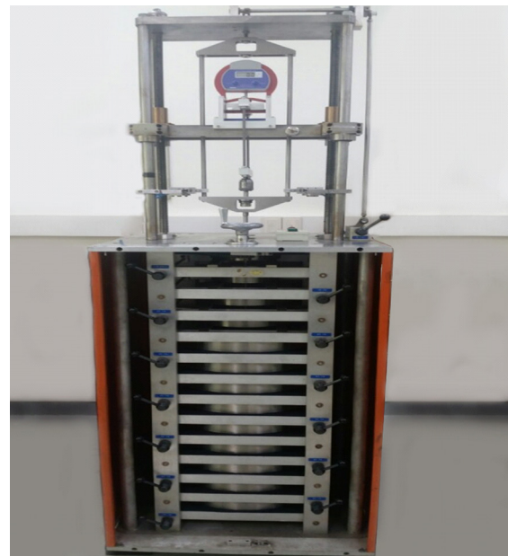
Fig. 4. Calibration by Actual Load Force Standard.
