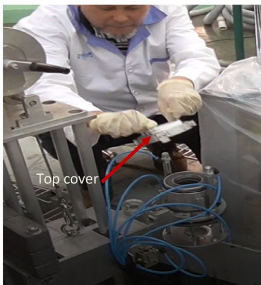
Fig. 13. Collimator cap is unscrewed and removed.
