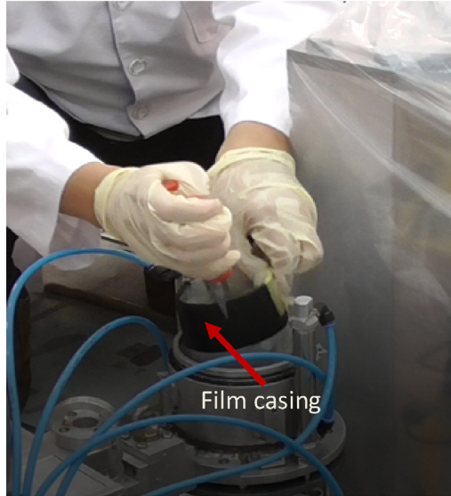
Fig. 15. Film is inserted into the compartment.
