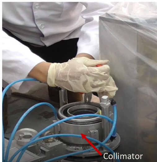
Fig. 16. It is important to ensure the film is properly position inside the compartment.
