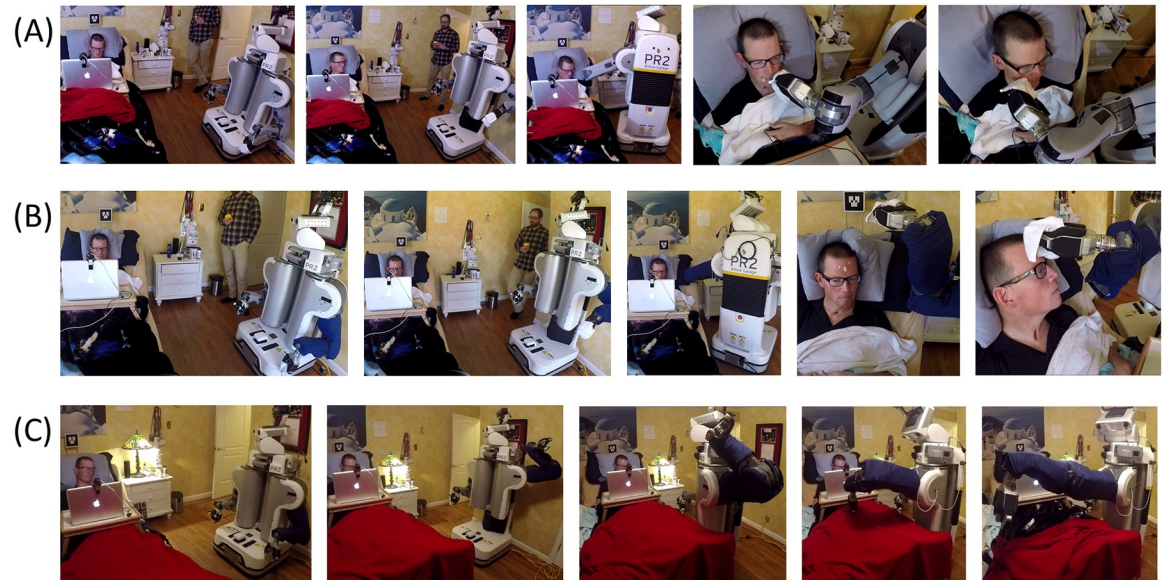
Fig 10. Image sequences from the three tasks performed by Henry. Using this system, Henry Evans was able to (A) wipe yogurt from his mouth, (B) wipe lotion from his forehead, and (C) pull a blanket down from his knees to his feet.
