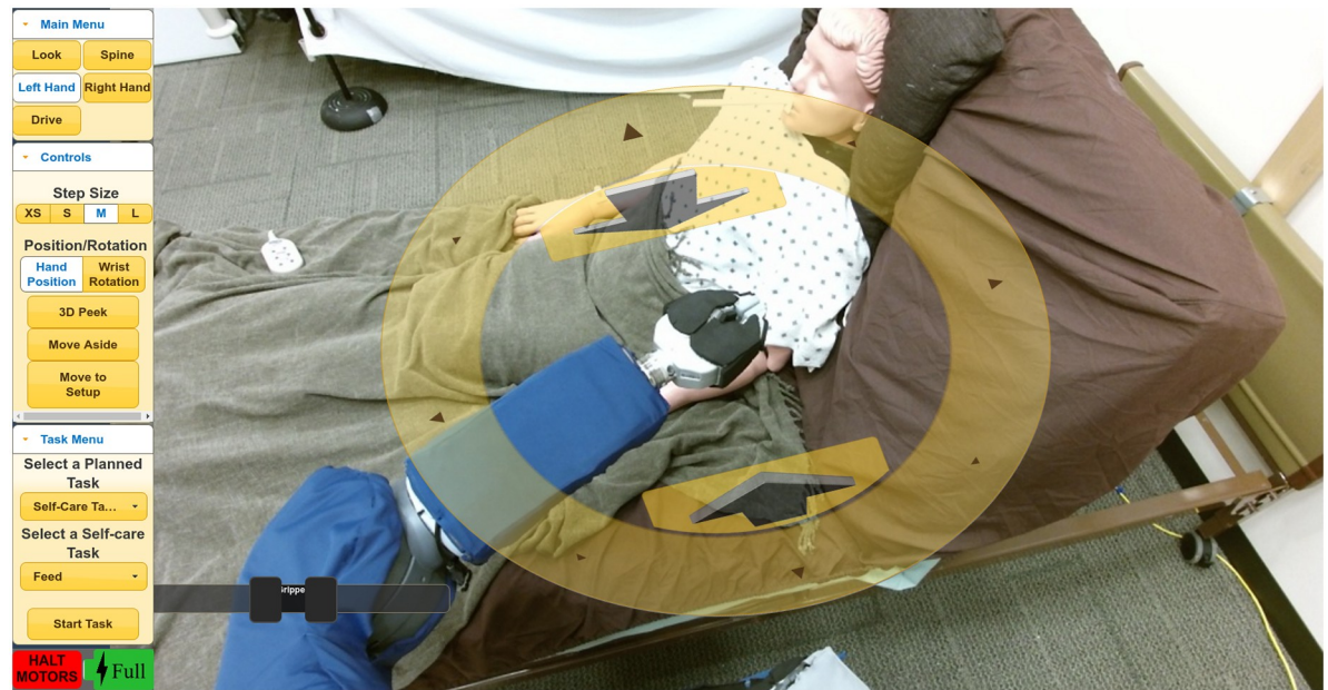
Fig 3. The web-based user interface. This interface enables low-level teleoperation by the user as well as the selection of autonomous planned tasks. Control modes and autonomous functions can be selected via buttons on the left.
