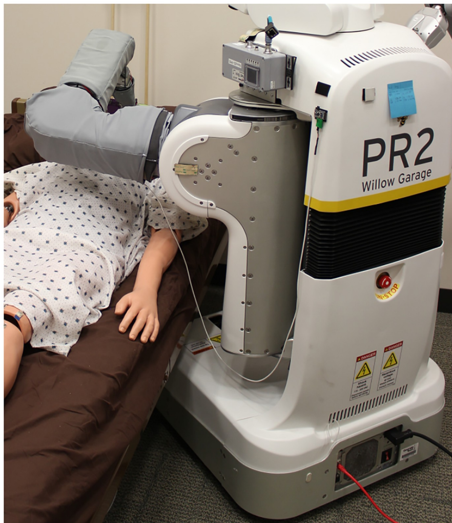
Fig 9. Physical collaboration between the two robots. A solution frequently used by the system was to raise the bed and to move the PR2's base under it, so the PR2 could better reach task areas.
