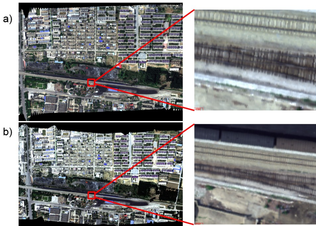
Figure 20. RGB synthesis image at high spatial/spectral resolution mode. (a) is high spatial mode (instantaneous field of view (IFOV) = 0.125 mrad) and (b) is high spectral mode (IFOV = 0.25 mrad).
