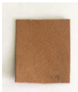
Figure 1. Undyed sample of vegetable tanned goat leather.
