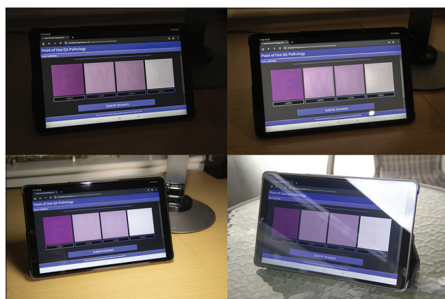
Figure 1: Photographs of the Point-of-Use Quality Assurance tool using a 10.1" Samsung Galaxy Tab A tablet under different lighting conditions. The device has a resolution of 1920 × 1200 pixels and a color depth of 16 million, with brightness set to maximum. Top left: unlit indoor environment. Top right: Artificially, indirectly lit indoor environment. Bottom left: Artificially, directly lit (LED lamp). Bottom right: Outdoor environment. All pictures use the same target letters: F, W, N, and T. The environment has a noticeable impact on the visibility of the letters
