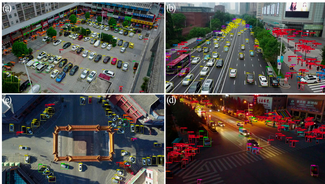
Figure 8. Partial test results obtained with Mixed YOLOv3-LITE using VisDrone2018-Det Val dataset. (a) Static object image, (b) dynamic object image, (c) orthographic image, and (d) bad light image.
