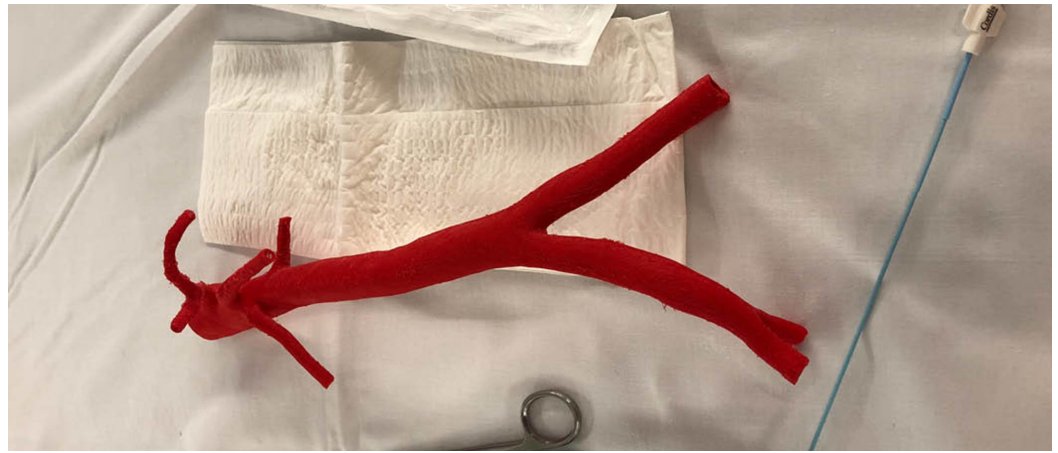
FIGURE 8: 3D-printed abdominal aorta using TPE 80A filament
