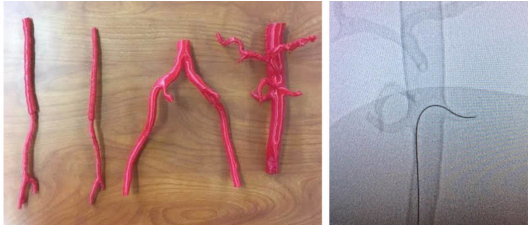
FIGURE 4: Vasculature models produced using NinjaFlex on a Lulzbot Taz 3D printer
