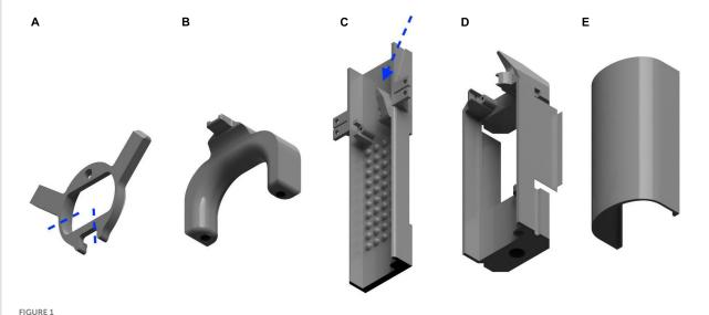
3D designs for awake-restrained imaging. (A) Frontal head holder with markers (blue) for cutting to allow space for the collar; (B) Collar head holder for neck stabilization. Holes in the base are threaded prior to surgery for fixation to the bed using plastic screws; (C) MRI imaging bed with air-puff applicator (blue arrow); (D) Optical imaging bed; (E) Lid for optical imaging bed.
