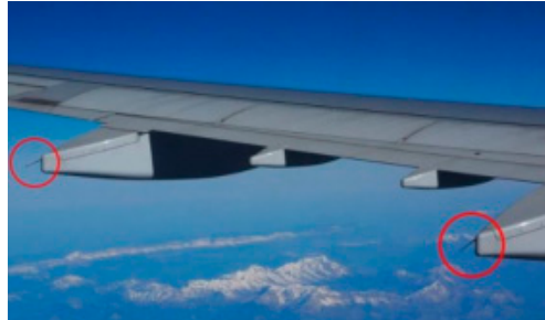
Figure 1. An aircraft can resume its flight safely because of the static dischargers (red circles) attached to its wings to discharge the electric current into the air.
