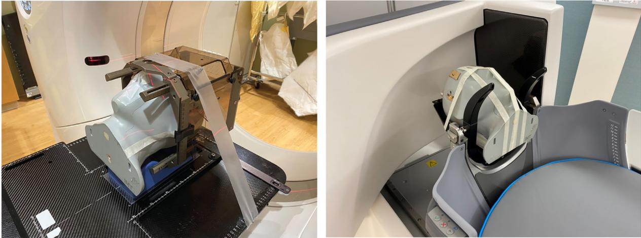
**FIGURE 3** Photos of tested G-Frame (left) and frameless (right) setups for E2E testing
