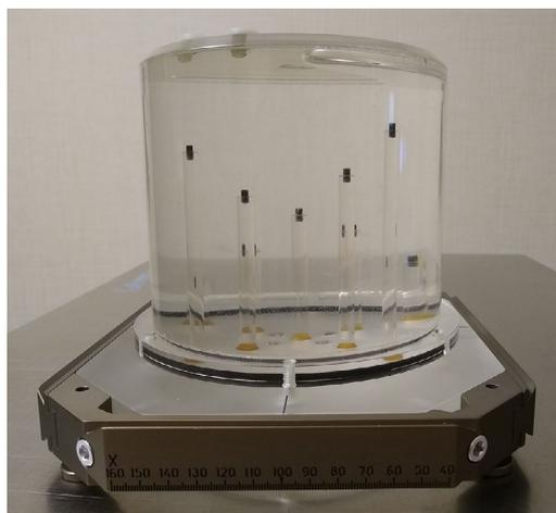
**FIGURE 1** Photograph of the in-house candlestick phantom
