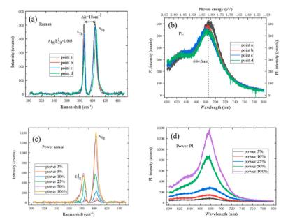
**Figure 2.** (a) The Raman spectrum of monolayer  $MoS_2$  at the different test points; (b) the PL spectrum of monolayer  $MoS_2$  at the different test points; (c) the Power Raman spectrum of monolayer  $MoS_2$ ; and (d) the Power PL spectrum of monolayer  $MoS_2$ .
