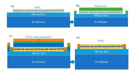
**Figure 3.** The main preparation process schematic diagram of the monolayer MoS<sub>2</sub>-based field effect transistor (FET; (**a**)) the growth process of the high-quality triangular monolayer MoS<sub>2</sub>; (**b**) the photolithography and the Ar plasma etching process; (**c**) the electron beam evaporation process; and (**d**) the cleaning process of the photoresist.
