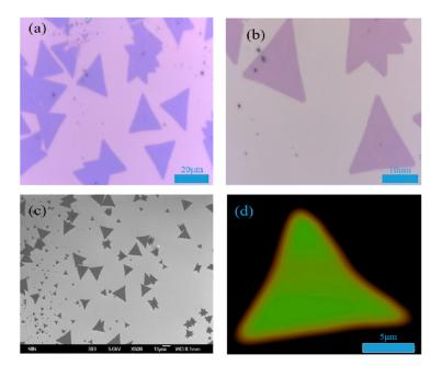
**Figure 1.** (a) The  $50\times$  objective optical micrograph of monolayer MoS<sub>2</sub>; (b) the  $100\times$  objective optical micrograph of monolayer MoS<sub>2</sub>; (c) the FESEM image of triangular monolayer MoS<sub>2</sub>; and (d) the mapping diagram of monolayer MoS<sub>2</sub>.
