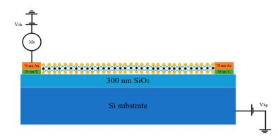
Figure 5. The electrical test structure of the monolayer MoS<sub>2</sub>-based back-gate FET.
