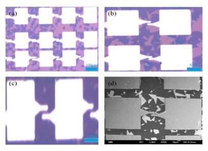
**Figure 4.** (a) The 10× objective optical microscope image; (b) the 50× objective optical microscope image; (c) the 100× objective optical microscope image of the monolayer MoS<sub>2</sub>-based back-gate FET; and (d) the FESEM image of the monolayer MoS<sub>2</sub>-based back-gate FET.
