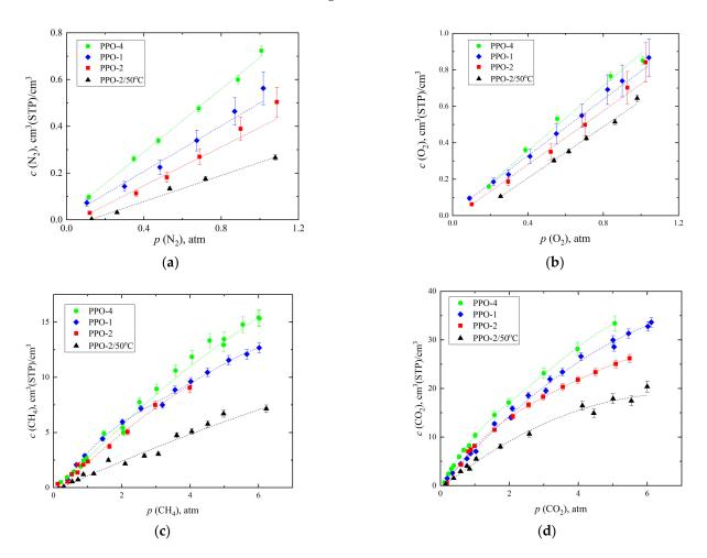
**Figure 6.** Sorption isotherms of  $N_2$  (a),  $O_2$  (b),  $CH_4$  (c), and  $CO_2$  (d) obtained by the volumetric method with chromatographic detection for PPO-2/50 °C, PPO-1, PPO-2, and PPO-4 film samples.
