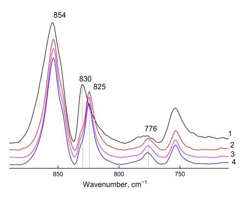
**Figure 3.** Fragments of ATR-FTIR spectra of PPO-2/50 °C (curve 1), PPO-1 (curve 2), PPO-4 (curve 3), and PPO-2 (curve 4) films in the vibrations absorption region characterizing the amorphous and crystalline phases (ZnSe crystal).
