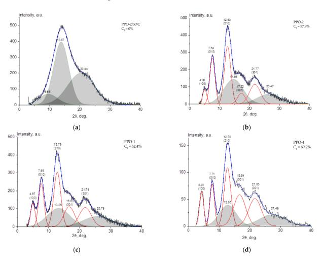
**Figure 2.** Diffractograms of PPO film samples with peak deconvolution. Grey peaks represent an amorphous phase. Red line peaks correspond to the peaks crystalline phase, blue line is a sum of the red peaks. Values over the peaks of crystalline phase are d-spacings and Miller indices (in parentheses). (a) PPO-2/50 °C film ( $C_I = 0\%$ ); (b) PPO-2 film ( $C_I = 57.9\%$ ); (c) PPO-1 film ( $C_I = 62.4\%$ ); and (d) PPO-4 film ( $C_I = 69.2\%$ ).
