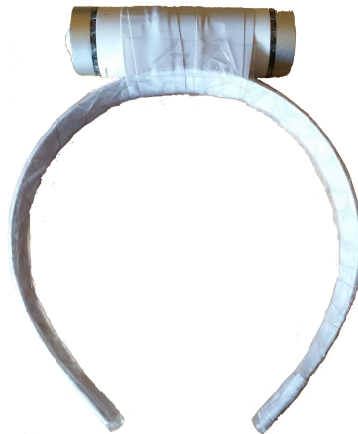
Figure 2. Node + sensor platform setup for head tremor assessment.
