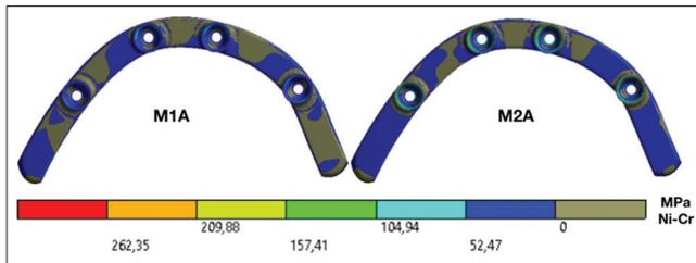
**Figure 7:** Maximum main stress under load on all teeth on nickel-chromium and polyether ether ketone bars (apical view-A)
