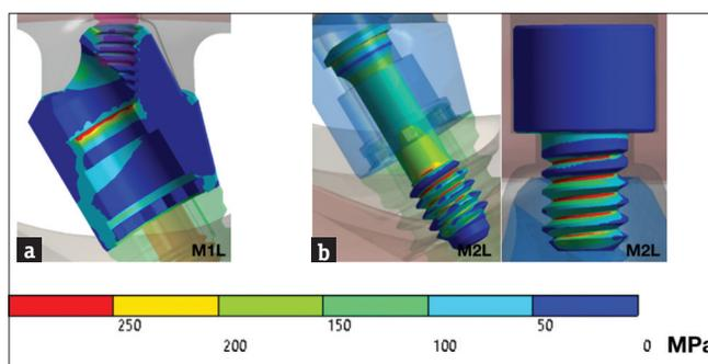
Figure 5: (a) Results of the left posterior implant under load for all teeth (lingual view-L). (b) Results for the intermediate's screw and left posterior screw under oblique load (lingual view-L)
