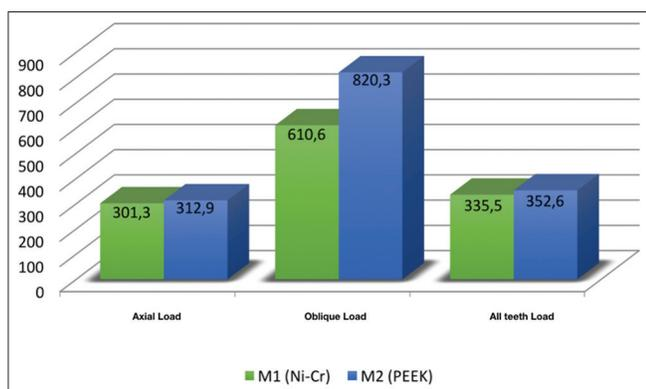
Figure 3: Peak stress on implants according to von Mises criterion (in megapascals)
