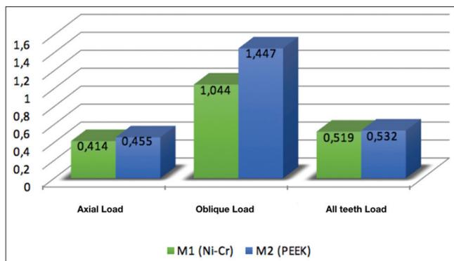
Figure 1: Peaks on peri-implant bone according to Mohr Coulomb criterion (in megapascals)
