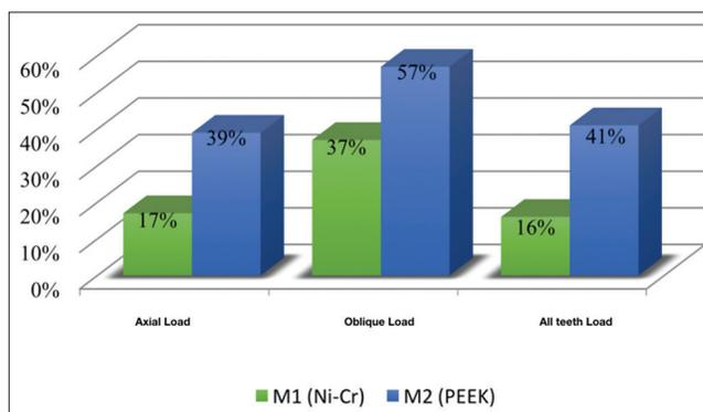
Figure 6: Percent of tensile yield strength on the outer sides peaks of the bars according to Rankine criterion (in megapascals)
