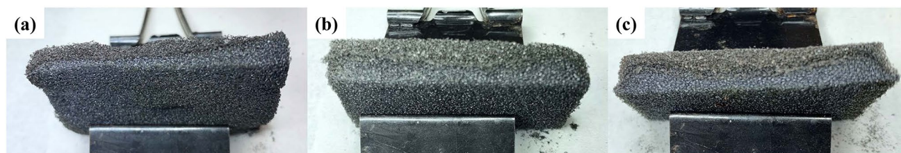
Figure 5. Cross-section digital images of UL-94 horizontal burning testing residues of (a) [CH/Casein/Ti 3 C 2 ] 2 , (b) [CH/Pectin/Ti 3 C 2 ] 2 , and (c) [CH/PA/Ti 3 C 2 ] 2 coated PUFs.
