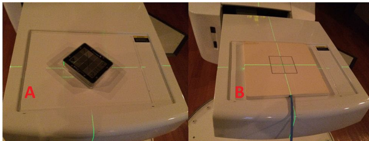
FIG. 3. The a-Si EPID flat-panel detector is shown with the (a) QC-3 image-quality phantom and (b) PTW975 Semiflex Ion Chamber and Plastic Water in measurement position.
