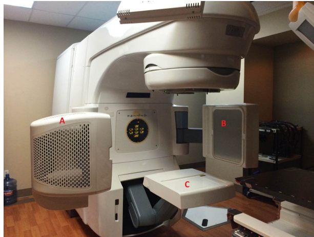
FIG. 1. The on board image (OBI) guidance system and EPID image system of the Varian Novalis Tx radiation delivery system are shown: (a) kV X-ray source of the OBI, (b) a-Si flat-panel detector of the OBI, and (c) MV a-Si EPID mounted to an ExactArm.
