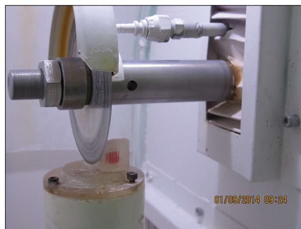
Figure 3: The composite specimen (red) merged in transparent acrylic resin.
