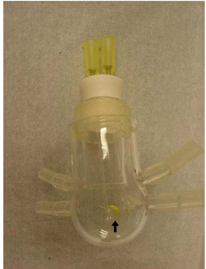
Figure 2. The culturing system. The arrow (→) indicates the IOL in culturing. Only one IOL was shown.
