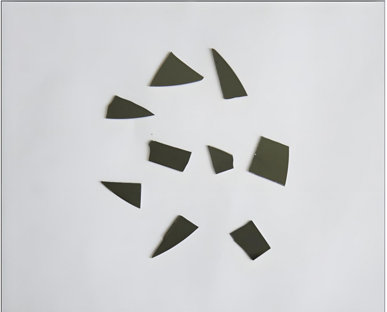
Fig 2. Mica chips for sample immobilization in AFM.
