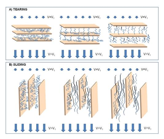
**Figure 20.** Proposed mechanisms (i.e., (**A**) tearing and (**B**) sliding) of elongational-flow-induced deformation of the tactoids in polymer/clay nanocomposites. Adapted with permission from Reference [218]. Copyright (2008) WILEY-VCH Verlag GmbH & Co. KGaA.
