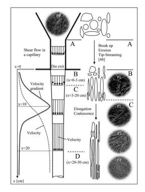
**Figure 16.** Mechanisms of fibrillation process along the spin line for a PLA filament. Reprinted with permission from Reference [167]. Copyright (2014) Elsevier.
