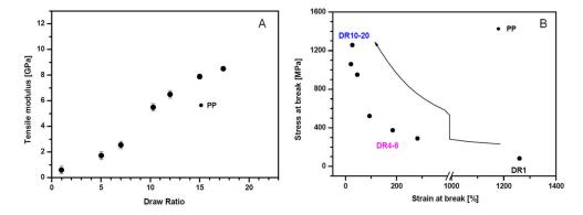
**Figure 9.** (**A**) Tensile modulus as a function of DR for melt-spun PP fibers, (**B**) stress at break as function of strain at break of selected PP fibers at different DR. Adapted from Reference [109] under CC BY 4.0 license.
