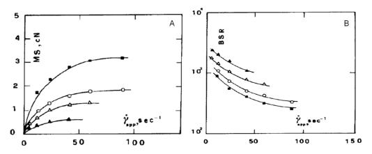
**Figure 5.** Melt strength (**A**) and breaking stretching ratio (**B**) as a function of shear rate for linear low-density polyethylene samples with different molecular weights. Reprinted with permission from Reference [67]. Copyright (1985) The Society of Rheology.
