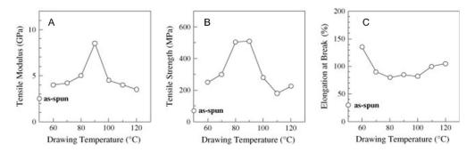
**Figure 12.** (**A**) Tensile modulus, (**B**) strength and (**C**) elongation at break of PLA fibers drawn at various temperatures. Reprinted with permission from Reference [126]. Copyright (2006) Elsevier.
