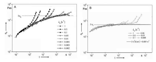
**Figure 6.** Temporal evolution of the elongational viscosities for (**A**) LDPE and (**B**) LLDPE samples at 150  $^{\circ}$ C and different elongational rates. Reprinted from Reference [41] under CC BY license.
