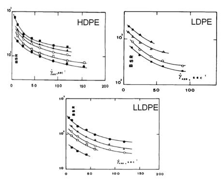
**Figure 8.** BSR values as a function of the shear rate for HDPE, LDPE and LLDPE samples with different molecular weights. Reprinted with permission from Reference [88]. Copyright (1985) WILEY-VCH Verlag GmbH & Co. KGaA.
