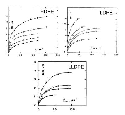
**Figure 7.** MS values as a function of the shear rate for HDPE, LDPE and LLDPE samples with different molecular weights. Reprinted with permission from Reference [88]. Copyright (1985) WILEY-VCH Verlag GmbH & Co. KGaA.
