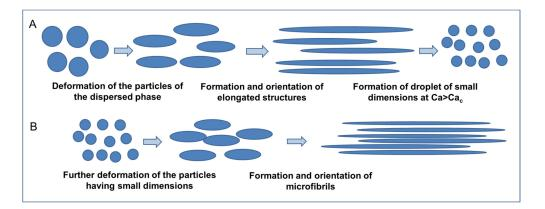
**Figure 15.** Schematic representation of the possible mechanism of the droplet-to-fibril transition in immiscible blends subjected to elongational flow: (**A**) Deformation of the original particles of the dispersed phase and (**B**) formation of microfibrillar structures.
