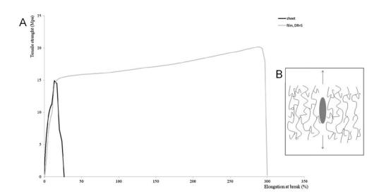
**Figure 18.** (**A**) Stress–strain curves of isotropic and anisotropic LDPE/PA6 samples and (**B**) sketch of the stress–strain test of the anisotropic film in MD. Reprinted with permission from Reference [34]. Copyright (2014) Elsevier.
