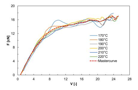
**Figure 4.** Rheotens curves for an LDPE sample obtained at different temperatures, and Rheotensmastercurve. Adapted with permission from Reference [66]. Copyright (1996) WILEY-VCH Verlag GmbH & Co. KGaA.
