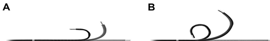
Fig. 3 The deflected radius of the 180-degree upward arm is shorter than that of the downward 275-degree arm, and acted with more agility. (A) 180-degree deflection; (B) 275-degree deflection.
