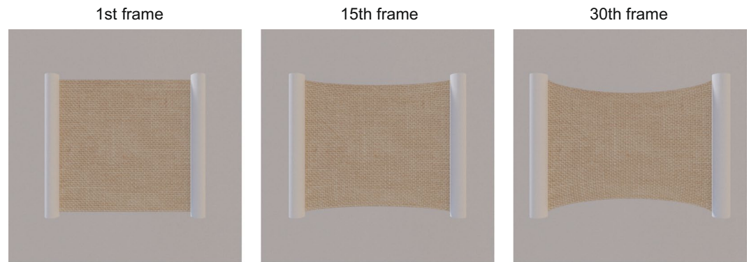
Figure 1. Snapshots of the video clip which simulates a horizontally stretched cloth by using Blender ( https://www.blender.org/ ). As the cloth is horizontally extended across video frames, vertical compression of the cloth occurs.
