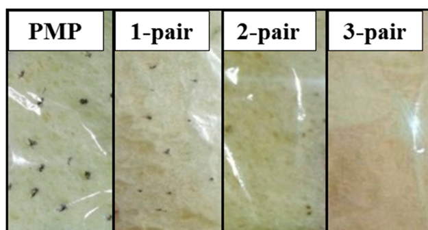
Figure 6. Images of food packed by PMP without and with different pairs of \text{SiO}_x/\text{SiC}_x\text{H}_y stacked film.
