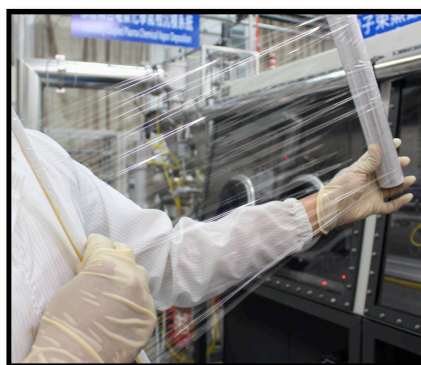
Figure 7. Photograph of stretched and rolled PMP with three-pair \text{SiO}_x/\text{SiC}_x\text{H}_y stack.
