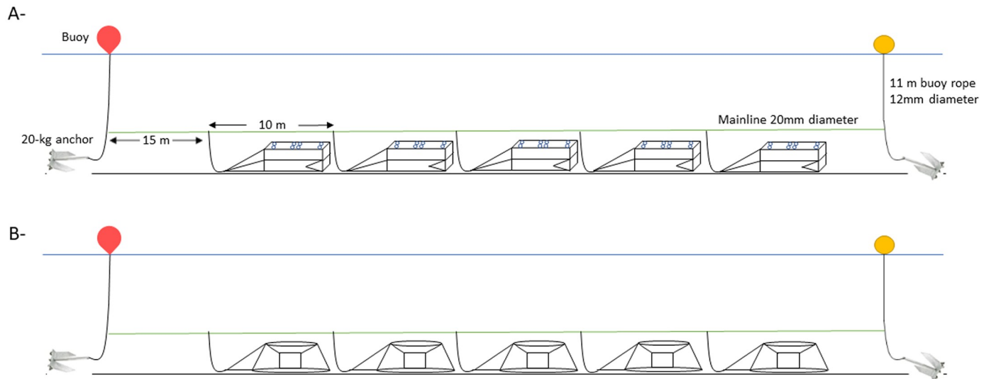
Fig 1. The two configurations tested. A- fishing line of lightweight traps, B- fishing line of heavy traps.
