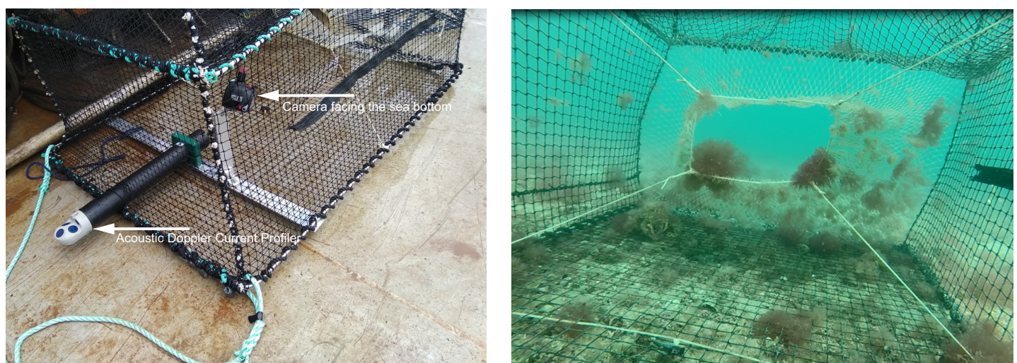
Fig 4. Position of the camera facing the sea bottom and of the Acoustic Doppler Current Profiler (left panel) and View of the bottom from the camera set to quantify the swept distance during retrieval (right panel).
