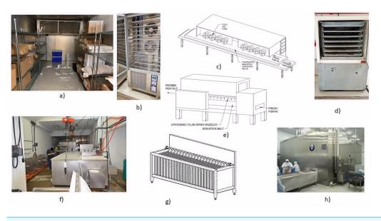
Figure 3 Examples of freezing systems: (A) Still air, (B) air blast, (C) tunnel, (D) horizontal plate, (E) cryogenic, (F) brine immersion, (G) vertical plate, and (H) spiral. Photo and drawing credits: Pete Brown.
