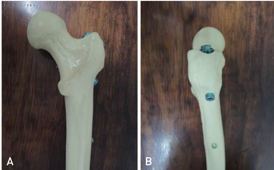
Fig. 1. Proximal femoral nail antirotation nail and a helical blade inserted into the femur replica. (A) Anteroposterior and (B) lateral views.
