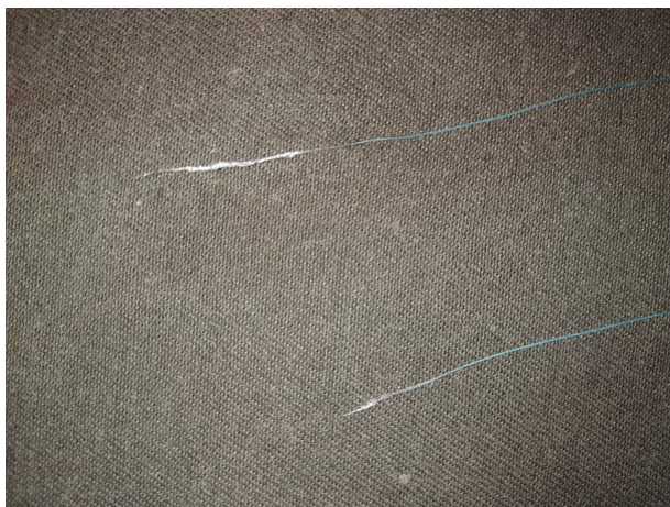
Figure 3 Examination of the broken tether showed damage, probably caused by abrasion.
