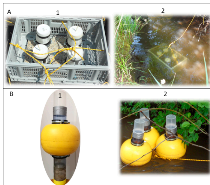
Figure 2. Photographs of active biomonitoring devices dedicated to in situ exposure of Chironomus riparius larvae. (A): submerged cages dedicated to the assessment of growth, survival and bioaccumulation; (B): Floating cages dedicated to the monitoring of emergence; 1: before deployment and 2: installed devices.
