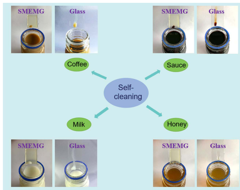
Fig. 5 Snapshots showing the sliding motion of coffee, sauce, milk, and honey droplets ( \sim 20 \mu\text{L} ) on the SMEMG and glass.
