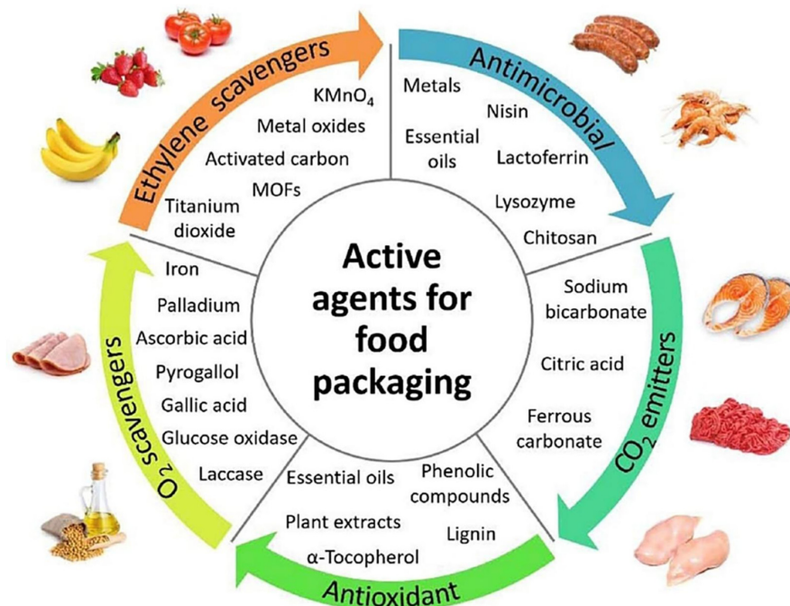
Figure 17. Bioactive agents for smart food packaging. Reprinted with permission from Elsevier, 2020 [303].
