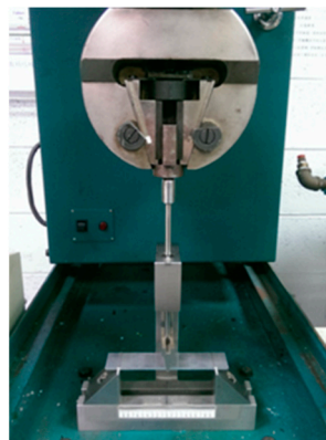
Figure 6. Experimental setup of the three-point bending test.
